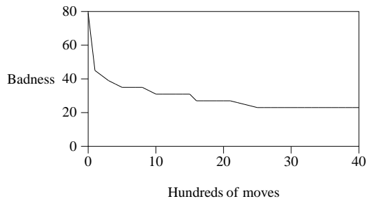
Fig. 7 Performance of tabu search on a typical teacher assignment problem ( bghs93 from Kingston 2008) with 305 teacher slots totalling 1275 times. The badness measure was the total number of clashes and hard workload limit overloads. After 4000 moves, starting from an initial greedy solution with badness 79, the best solution found had badness 23. The neighbourhood was all moves of one assignment from one qualified teacher to another. A move was tabu if its slot had been moved recently; the tabu list length was 50, which gave the best result of about ten values tried.
