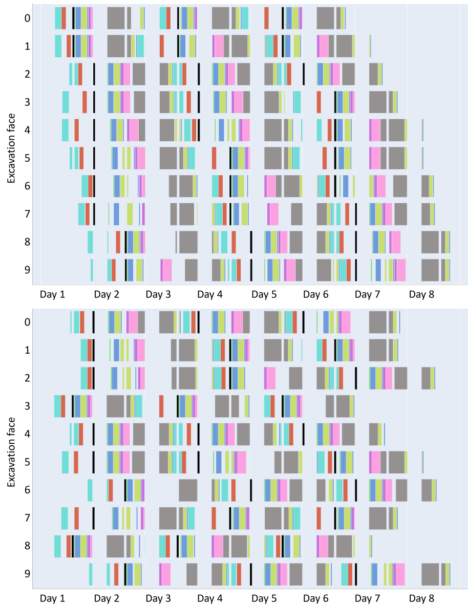
Fig. 2. Schedules for instance 10F:3C for the priority order P1 (order: 1,2,3,4,5,6,7,8,9,10) and P2 (order: 4,9,6,5,1,8,3,2,7,10), respectively. Colours are: turquoise for drillrigs 1-2, red for chargers 1-2, green for watering trucks 1-2, blue for loaders 1-5, lime green for scalars 1-3, purple for shotcreters 1-2, grey for bolters 1-4, and pink for afterlag
