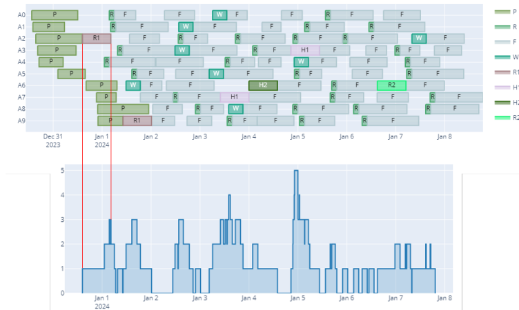
Fig. 1: Solution visualization: Aircraft on top, combined maintenance below
